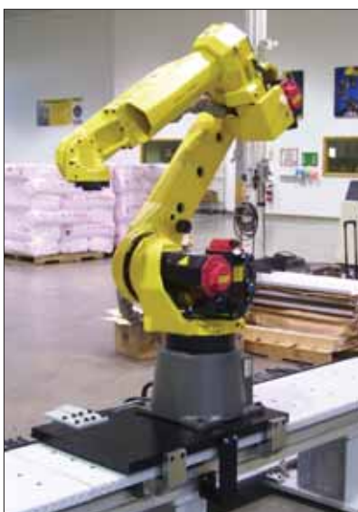
Fig 5 Big Sky's new robot under construction – the rail on which it sits is the 7th axis
