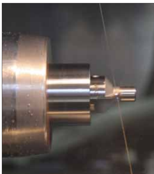
Fig 6 A countersink tool for use in the aerospace industry is cut on a Probe rotary machine
