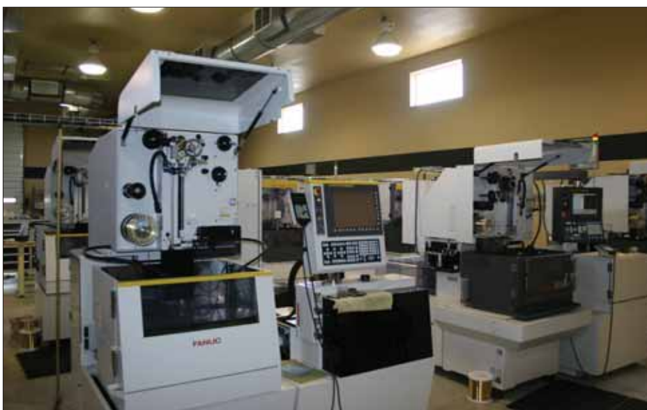
Figures 1 and 2 Big Sky now has 10 wire EDM machines for cutting PCD and PCBN discs
