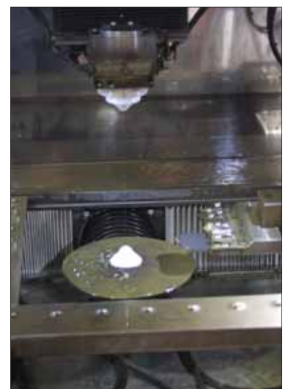
Fig 7 A Fanuc wire EDM cutting small triangles from a 58 mm diameter PCD disc
